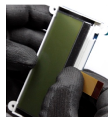
10-Fix and fit the centralized display
