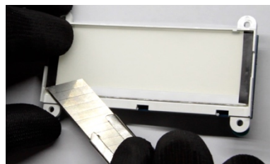
7-Fix the light masks to the edges
