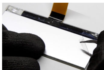
9-Remove the protective film
