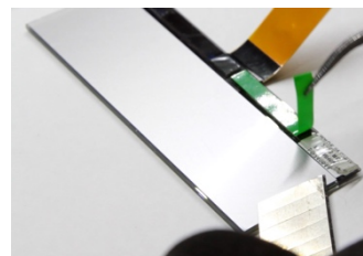
8-Use double-sided tape to secure the glass
